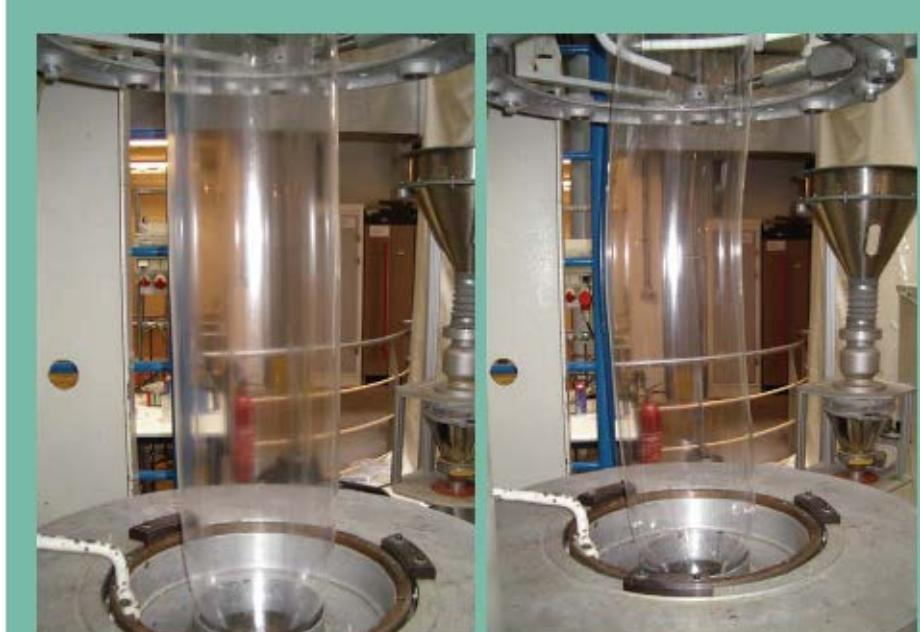
PLA film with (left) and without (right) Cesa-Extend from Clariant Masterbatches.
