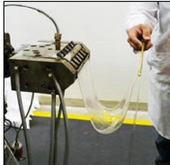
Arkema's Biostrength 700 **acrylic copolymer** has been shown to double the melt strength of PLA at 4% addition level (right) vs. a neat PLA (left).
