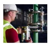
FLEXIBLE TO MEET THE JOB DEMANDS Thanks to the Acrobat's narrow jaw construction and compact package, flange-to-pipe, fitting-to-pipe and even fitting-to-fitting fusions can be done with ease.
