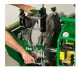
AVAILABLE HYDRAULIC CLAMPING Save time and increase productivity by eliminating manual-crank clamp knobs on 618 machines. To purchase, add "HC" to the end of the part number above.
