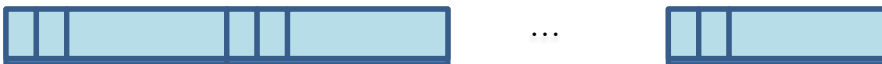
Figure 16: The PCM Packets are sent one after the other to the TCP Socket or to the Target log file.
