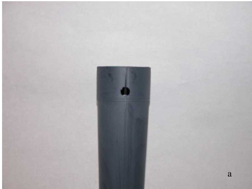
Appendix E-1. Photograph depicting a conetainer used in the indirect experiment with drilled hole and cut to allow for sprig to be inserted without tissue damage.
