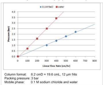
Fig. 1 Pressure-flow properties of POROS<sup>™</sup> XQ resin
