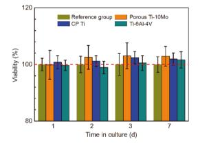
Figure 3 Effect of extracts of porous Ti-10Mo, CP Ti and Ti-6Al-4V alloy on viability of MC3T3-E1 cells at specific times of 1, 2, 3 and 7 days.
