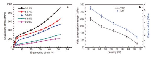
Figure 2 (a) Engineering stress-strain curves of Ti-10Mo alloys with different total porosities. (b) Influence of porosity on compression yield strength and elastic modulus of Ti-10Mo alloys.
