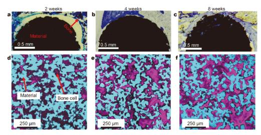
Figure 8 Histological section of porous Ti-10Mo alloy implant at different times of implantation: (a-c) optical micrographs, (d-f) fluorescence micrographs.
