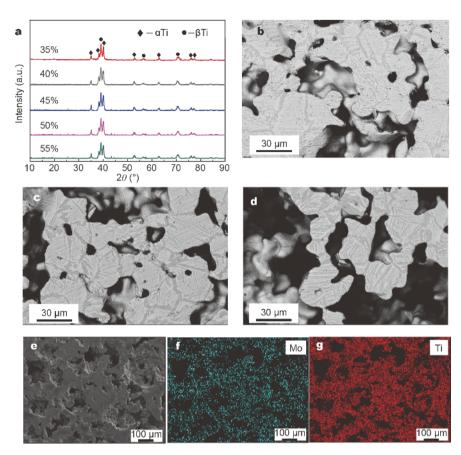
Figure 1 (a) XRD patterns, (b–d) SEM backscatter electron images showing microstructures of Ti-10Mo alloys with different weight ratios of spaceholder added: (b) 35%, (c) 45%, and (d) 55%, and (e–g) SEM secondary electron image of Ti-10Mo alloy with 35% space-holder added and corresponding mapping of Ti and Mo elements.
