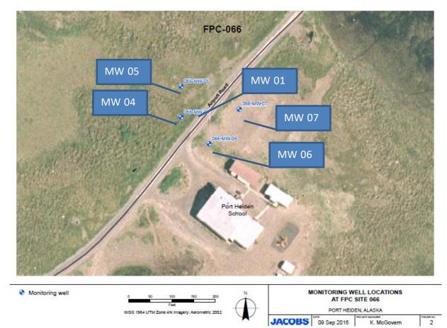
Figure 10. Pipeline Spill Monitoring Wells Near the School [USAF 2016b].
