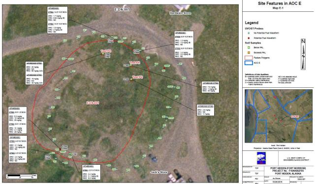
Figure 9. Sampling Locations Near Commercial Buildings in AOC E [USACE 2016]
