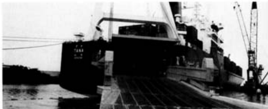
The M/V TANA is one of two roll-on/roll-off cargo vessels calling at U.S. and West African ports for Barber West Africa Line. Each ship is equipped with a stern-quarter ramp for the handling of RO/RO cargo and two 40-foot capacity deck cranes for handling containers.
