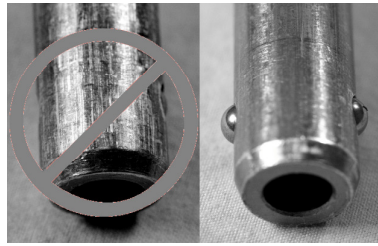
Fig 16 Left pin – retired due to wear and detent pins not properly working; Right pin – in good working condition
