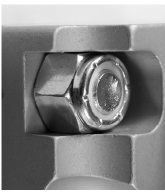
Fig 19 Bolt protrudes just beyond flush
