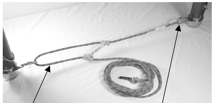
Fig 12 Rope Hobble Loop with Prussic. Sewn loop connected to quick link; large loop connected to 2 nd leg quick link.
