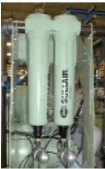
Primary and secondary filters with condensate trap remove particles and aerosols.
