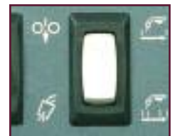
Inch and Gas purge switch
