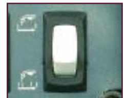
Gun trigger hold switch (2T/4T)
