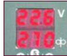
Digital display meter, wire feed speed (IPM or MPM), amperage, voltage, arc time and memory hold
