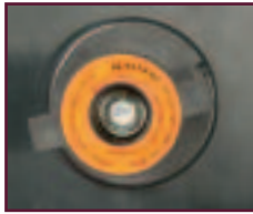
Wire spool hub with locking assembly
