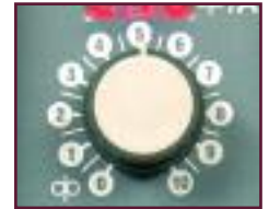
Wire feed speed dial with large rubberized control knob
