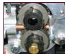
Quick change drive rolls, no tools required
