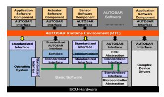
Figure 1: AUTOSAR layer structure
