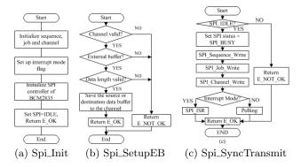
Figure 6: Flow charts of three SPI functions.
