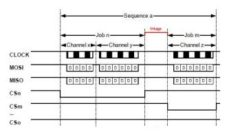
Figure 5: SPI transmission structure
