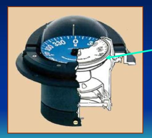
Gimbal system to keep card level when ship heels and pitches.
