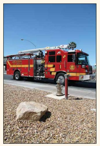
Step 1: Position apparatus a few feet (meters) short of hydrant. Chock wheels.
