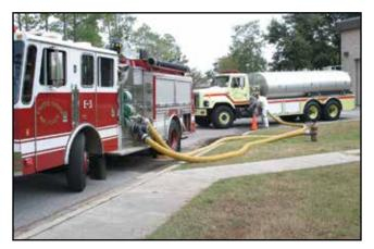
Figure 4.3 Lay supply hose to the side of the street from hydrant to pumper.
