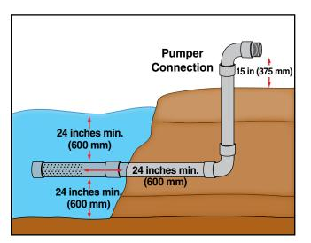
Figure 4.8 A dry hydrant installation.
