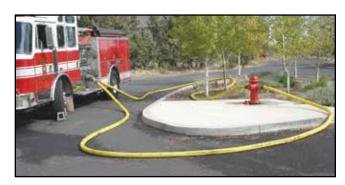
Figure 4.11 An apparatus connected to a hydrant using two 2½ inch (65 mm) hoselines.
