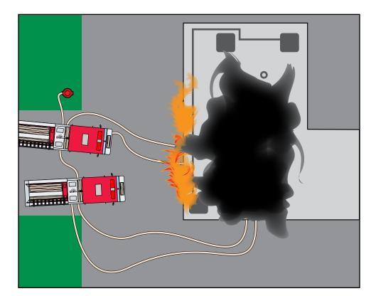
**Figure 4.12** Dual pumping operations.
