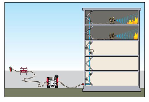
Figure 4.13 Tandem pumping operations.
