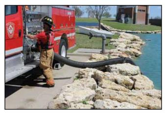
**Figure 4.7** A pumping apparatus set up for a drafting operation from a static water supply.
