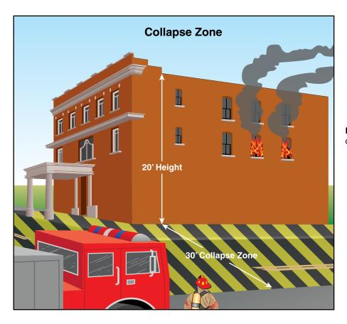
**Figure 4.4** Position the apparatus outside of the collapse zone.
