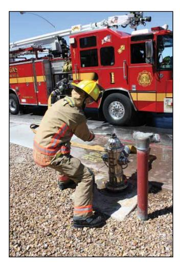
Side intake connections. To avoid blocking the street with the apparatus, the driver/operator must stop close to the curb with the pump intake a few feet short of being in line with the hydrant (Figure 4.10).
