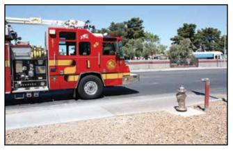
**Figure 4.10** The pumper is close to the curb and in proper position to make a hydrant connection.
