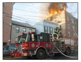
**Figure 4.5** Parking a pumper directly below a large number of utility lines may be dangerous, especially if fire or weather conditions cause them to fall. *Courtesy of Ron Jeffers.*  The driver/operator should also consider the ability to remove portable equipment from the apparatus. Therefore, park in a position where compartment doors may be fully opened and ground ladders or other portable equipment may be removed safely and efficiently from the apparatus.
