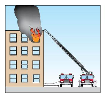
**Figure 4.6a** The aerial is positioned outside the pumper because the building is less than five stories tall.
