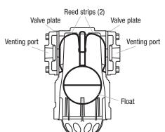
Float-actuated reed strips uncover vent holes in valve plates when vapor is present, effectively eliminating free air or vapor from the system before it can enter the meter. Reed strips seal off vent holes when liquid level rises in chamber
