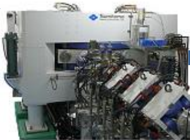
Sumitomi Heavy Industries Cyclotron 18 MeV protons, 50 \mu\text{A} beam current
