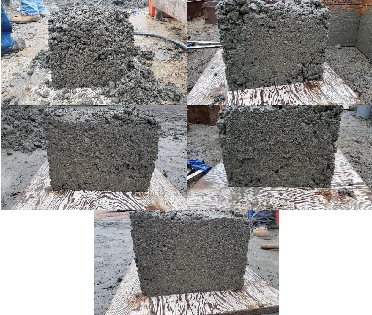
Figure 5 (a-e): Example Box Test results obtained during mixture development phase.
