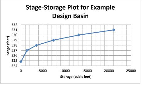
$\circ~$  The proposed pond's storage volume is sufficient to hold the WQ\_v, and is assumed to be sufficient for the other required peak flow controls.
