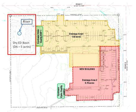
**Step 1** – Make a preliminary judgment as to whether site conditions are appropriate for the use of a dry pond or dry ED pond, and identify the function of the pond in the overall treatment system. This includes performing an initial suitability screening for the site.
