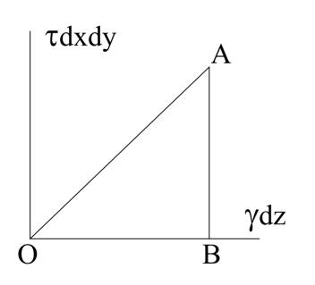
In general, if the body is subjected only to a *shear stress*  $\tau$ , the strain energy due to shear stress in the body is then
