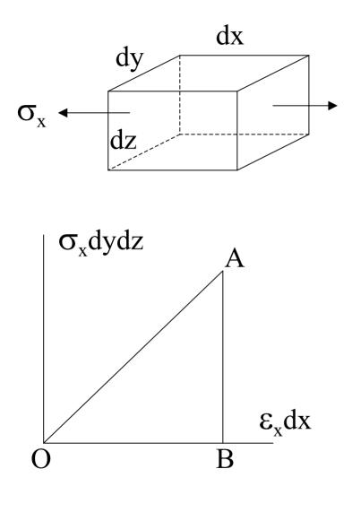
The force  $\sigma_x dydz$  does work on an extension  $\epsilon_x dx$
