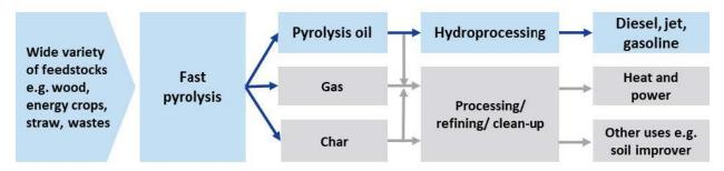
Figure 25. Value chain for fast pyrolysis with catalytic upgrading (O' Connell et al., 2019).
