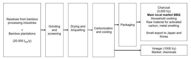
Figure 44. Block diagram. Charcoal briquette plant in Guande, China
