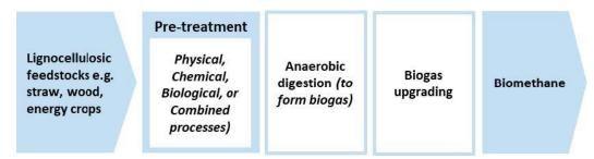
Figure 22. Value chain for AD with pre-treatment (O' Connell et al., 2019).
