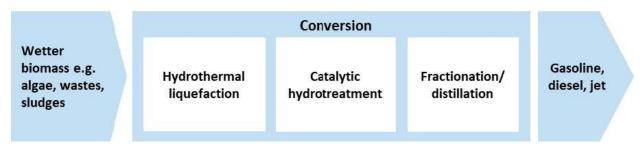
Figure 23. Value chain for HTL with catalytic upgrading (O' Connell et al., 2019).
