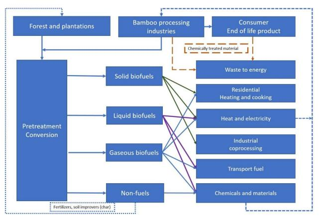
Figure 7. Schematic view of suitable bamboo streams for bioenergy production.
