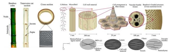
**Figure 14.** a. Macroscale anatomy of a bamboo culm. b. Hierarchical structure of bamboo and its micromechanical representation (Gangwar and Schillinger, 2019).
