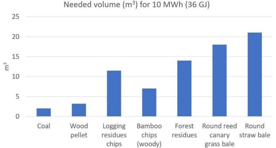
Figure 13. Energy density of relevant fuels.
