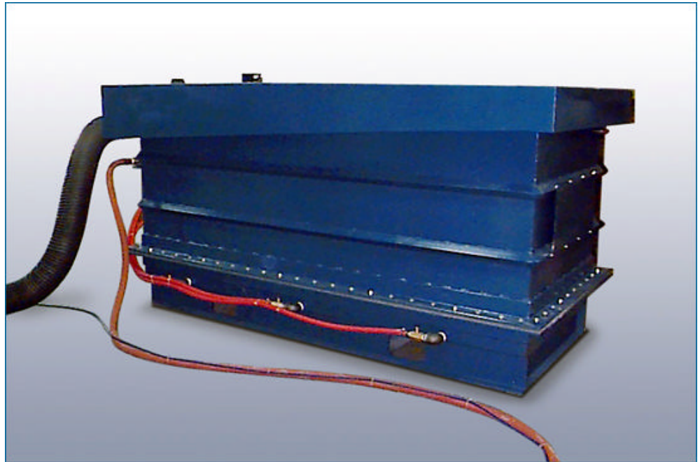
Typical fluidizing hopper used for applying powder coatings. Fluidizing hoppers can be as small as 1 lb or over 1000 lbs.
