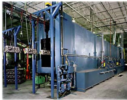
Example of a 5 stage washer system
