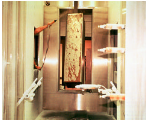
This is a part which is too dirty to be properly powder coated.
