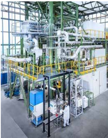
Picture 1: Full scale powder atomization plant in the 3D Competence Center at SMS group Germany
