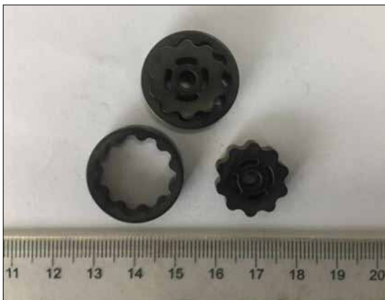
Figure 1. Gas nitrocarburized rotor produced by NBTM
