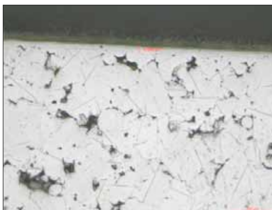
Figure 5. Metallographic of plasma nitrided small connecting rod
