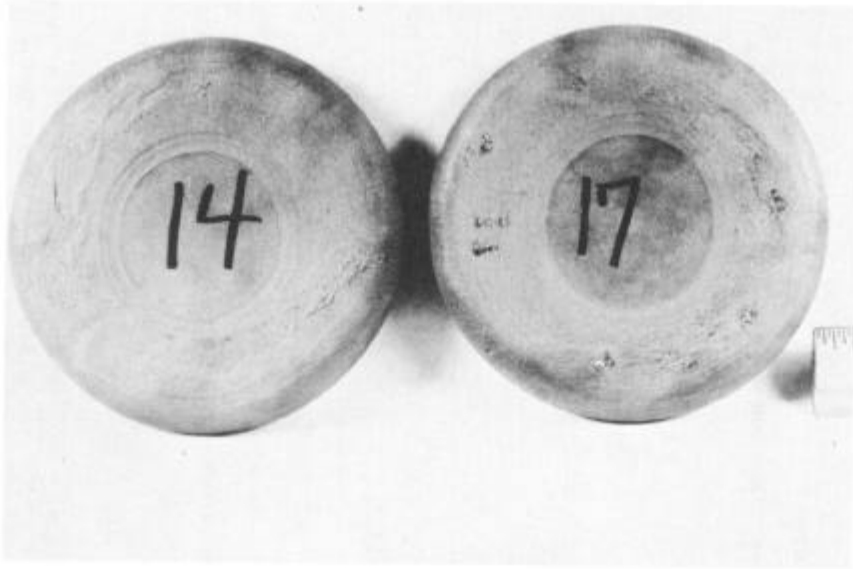
Figure 6: TYPICAL PA101 5 INCH DIAMETER PANCAKE FORGINGS
