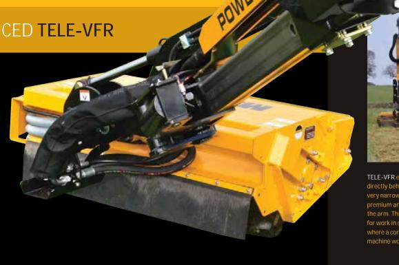
TELE-VFR enables operators to cut directly behind the cab when working in very narrow lanes where space is at a premium and there is no room to extend the arm. This creates opportunities for work in challenging environments where a conventional reach arm machine would struggle.
