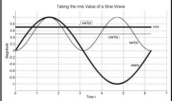
In an electrical circuit, rms terms are associated with heating or power. Given a voltage or current waveform, the rms value is obtain by 1) squaring the waveform, 2) finding the area under the waveform (integrating) over the length of one cycle, 3) dividing by the period, and 4) taking the square root of the result.
