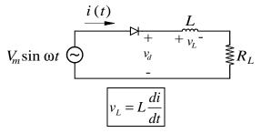
While current is flowing through the diode, there is zero voltage across the diode. When current flow stops at angle  $\beta$ , the voltage across the diode becomes negative (discontinuous). Since the average (dc) voltage at the source is zero and the average voltage across an inductor is zero, the average voltage across  $R_L$  is the negative of the average voltage across the diode.
