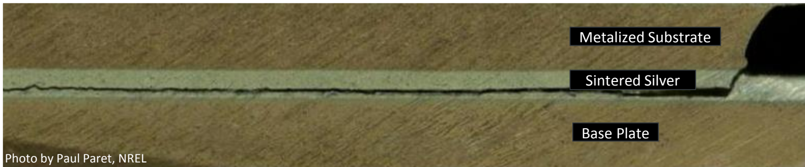
Crack Propagation in Pressure-Assisted (30 – 40 MPa) Sintered Silver
