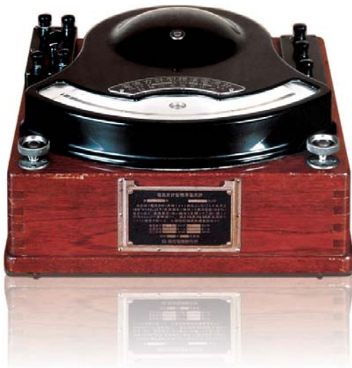
1930 Vintage Standard AC Voltmeter 0.2% Accuracy Class
