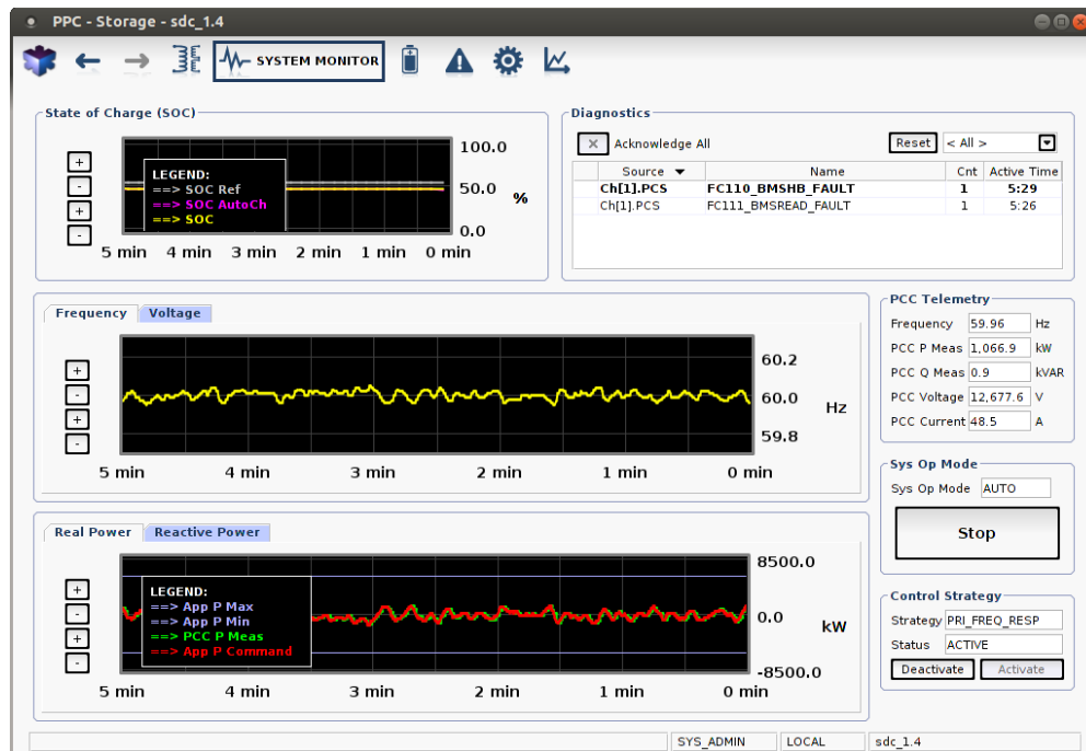
Figure 4: HMI screen snapshot - System monitor screen
