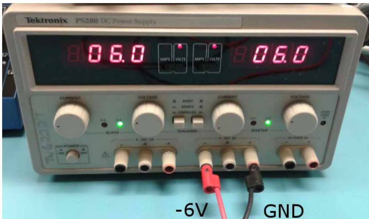
Figure 2: Single Negative Supply. The black lead is ground and the red lead is -6V.
