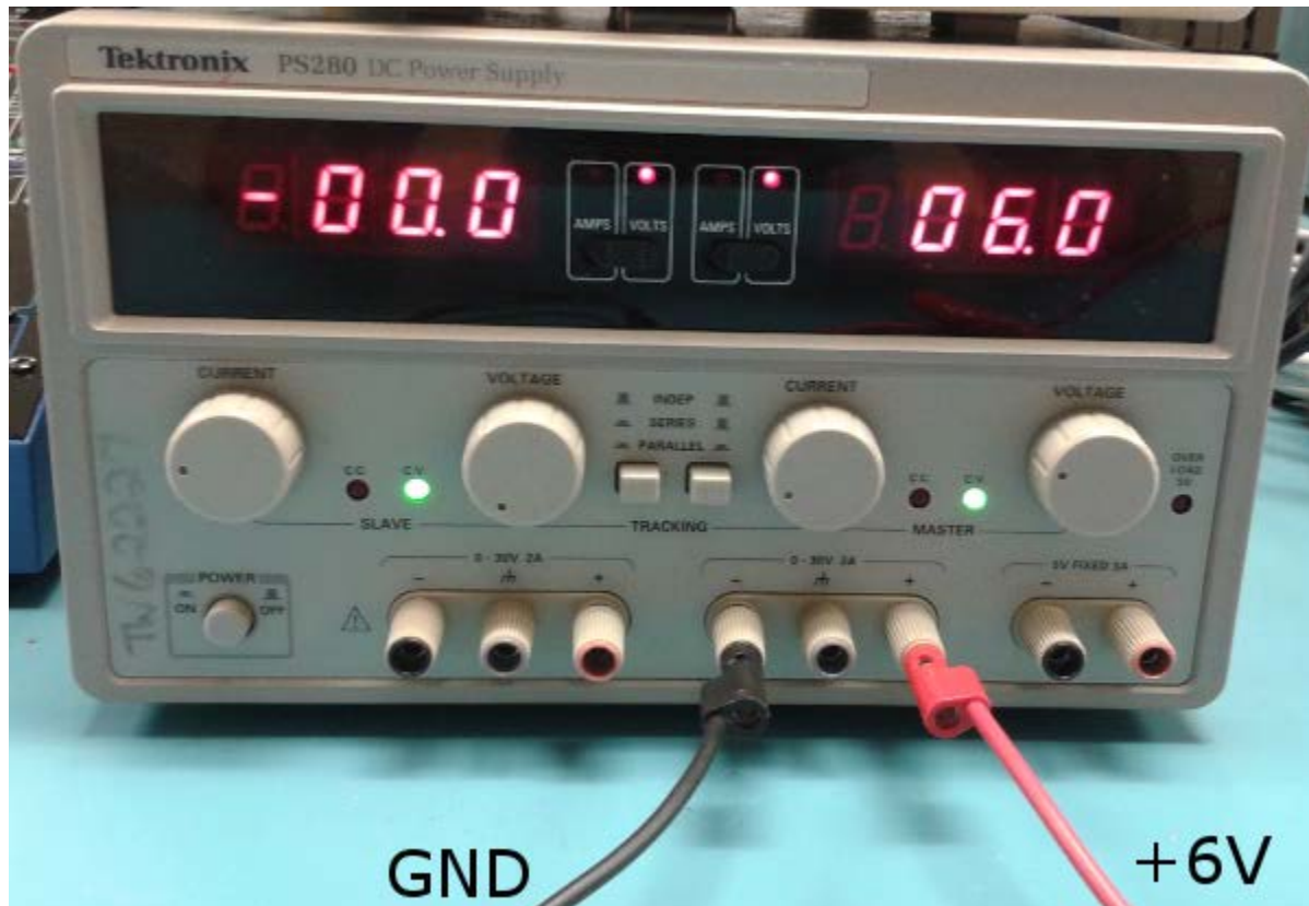
Figure 1: Single Positive Supply. The black lead is ground and the red lead is +6V.
