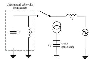
Figure. 9. Series resonance triggered by cable energization, adapted from [12]
