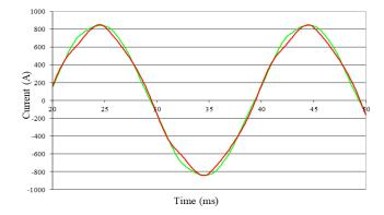
Figure. 5. Current through a 130/10 kV transformer before (green) and after (red) capacitor energization
