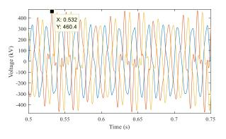
Figure. 8. Example of temporary overvoltages following transformer energization
