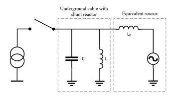
Figure. 6. Parallel resonance triggered by transformer inrush, adapted from [12]
