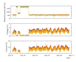
Figure. 4. Reactive power (top), 7th harmonic voltage (middle) and 7th harmonic current (bottom) following the connection of a capacitor bank
