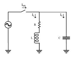
Figure. 1. Example circuit showing the energization of a compensated cable
