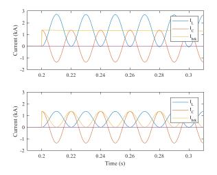
Figure. 2. Example of Zero Miss phenomenon, 100% (top) and 50% (bottom) compensation
