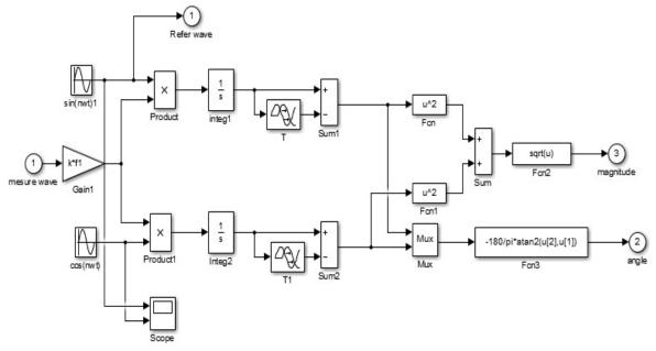
Figure 5: Basic Simulink Model of PMU
