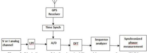
Figure 2: Block diagram of the Synchronized Phasor Measurement System (PMU)
