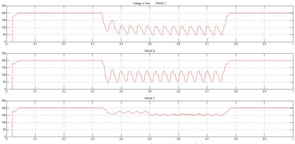
Figure 14: Voltage at bus no:4 during fault
