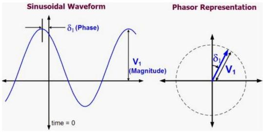
Figure 1: Phasor representation of sinusoidal signal
