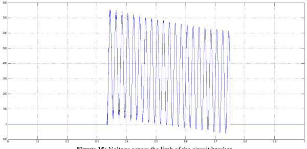
Figure 15: Voltage across the limb of the circuit breaker
