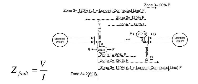
Distance protection is directional Relay is capable of multiple setting (Zones)
