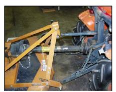
Figure 2. Driveline connected to the tractor
