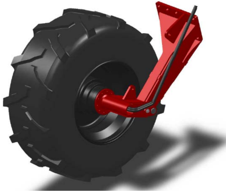
Figure A.1 – 3-D model of rear strut assembly with Black Bruin Motor
