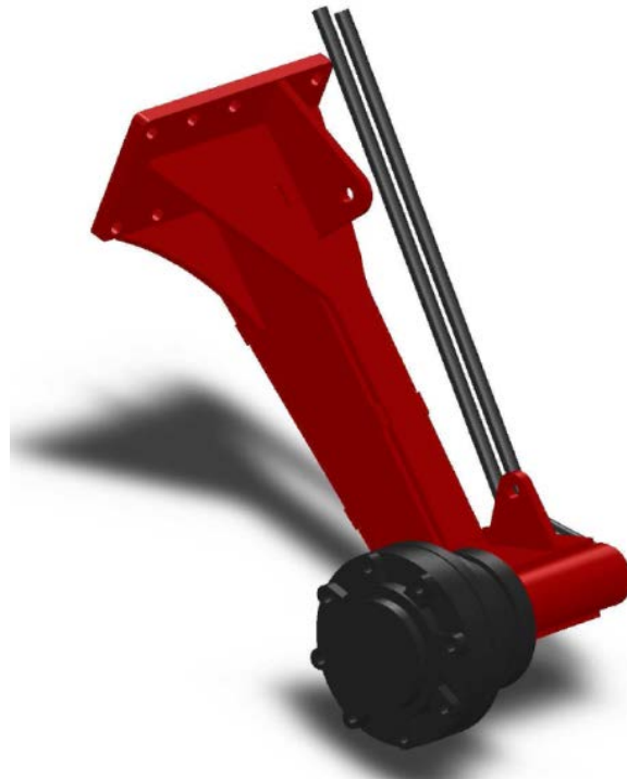
Figure A.2 – 3-D model of rear strut assembly without tire
