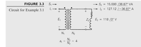
when the load voltage is 118 V. Assume that the transformer is ideal and calculate the following:
