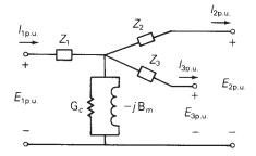
(c) Per-unit equivalent circuit-practical transformer
