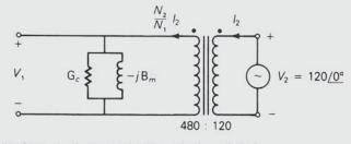
(b) Open-circuit test (neglecting series impedance)
