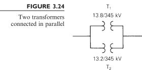
transformer  $T_1$  requires  $V_{baseX} = 13.8$  kV and  $T_2$  requires  $V_{baseX} = 13.2$  kV. It is clearly impossible to select the appropriate voltage bases for both transformers.
