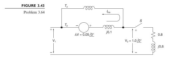
**3.65** Reconsider Problem 3.64 with the change that now  $T_b$  includes both a transformer of the same turns ratio as  $T_a$  and a regulating transformer with a 3° phase shift. On the base of  $T_a$ , the impedance of the two components of  $T_b$  is *j*0.1 per unit. Determine the complex power in per unit transmitted to the load through each transformer. Comment on how the transformers share the real and reactive powers.
