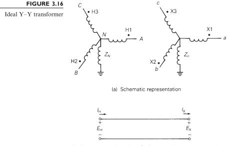
(b) Per-unit equivalent circuit for balanced three-phase operation
