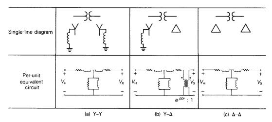
**FIGURE 3.17** Per-unit equivalent circuits of practical Y–Y, Y– $\Delta$ , and  $\Delta$ – $\Delta$  transformers for balanced three-phase operation
