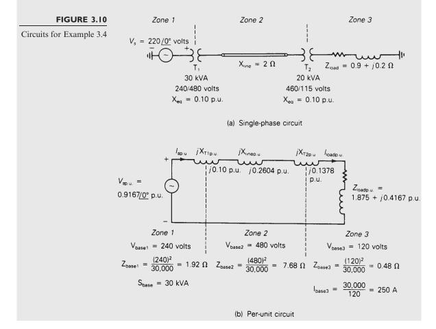
determine the per-unit impedances and the per-unit source voltage. Then calculate the load current both in per-unit and in amperes. Transformer winding resistances and shunt admittance branches are neglected.
