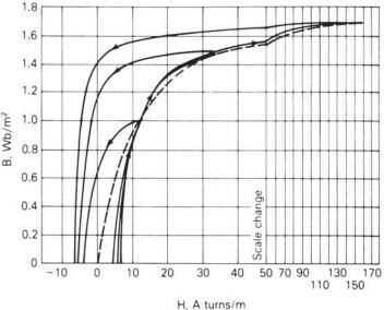
magnetizing current will flow. In a well-designed transformer, the applied peak voltage causes the peak flux density in steady state to occur at the knee of the B–H curve, with a corresponding low value of magnetizing current.
