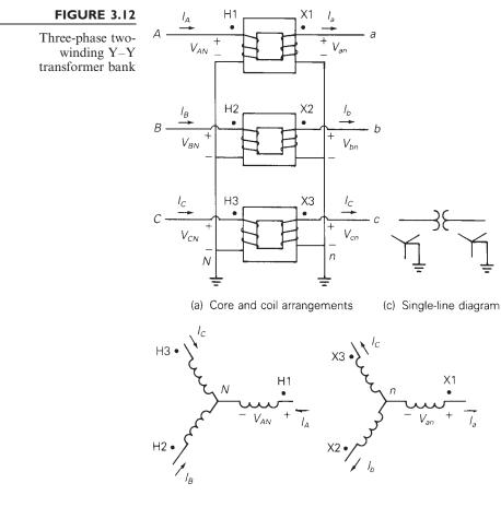
(b) Schematic representation showing phasor relationship for positive sequence operation
