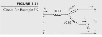
The per-unit equivalent circuit of this three-winding transformer is shown in Figure 3.21. Note that  $X_2$  is negative. This illustrates the fact that  $X_1$ ,  $X_2$ , and  $X_3$  are *not* leakage reactances, but instead are equivalent reactances derived from the leakage reactances. Leakage reactances are always positive.
