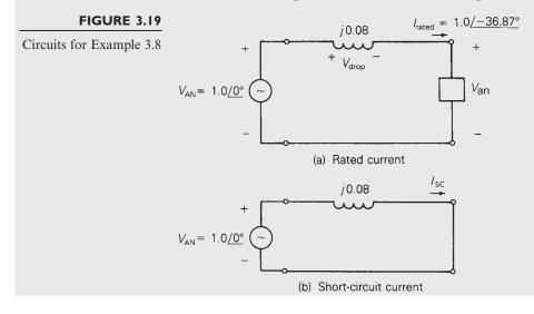
[part (b)], the fault current is 12.5 times the rated transformer current. This example illustrates a compromise in the design or specification of transformer leakage reactance. A low value is desired to minimize voltage drops, but a high value is desired to limit fault currents. Typical transformer leakage reactances are given in Table A.2 in the Appendix.
