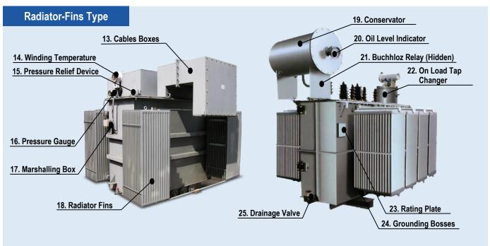
The following are the brief description of the main components typically found in an Oil Immersed Transformers:
