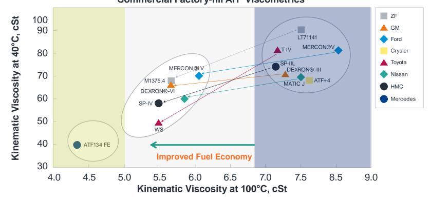
Some OEMs are replacing high-vis ATF with low-vis ATF
