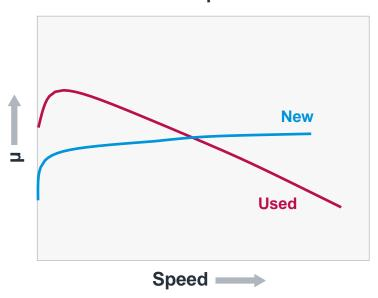
Reasonable  $\mu$  level with positive slope required
