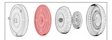
Torque Converter Lock-Up Clutch
