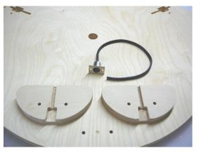
shows the foot halves at this position, although they are shown on top of the groundboard, in actuality they will be glued together and then to the <u>bottom side</u>.
