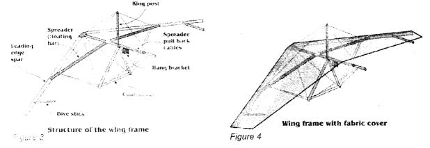
Nylon, Dacron and other modern fabric is attached firmly to the leading edge tubes (see figure 4). The
