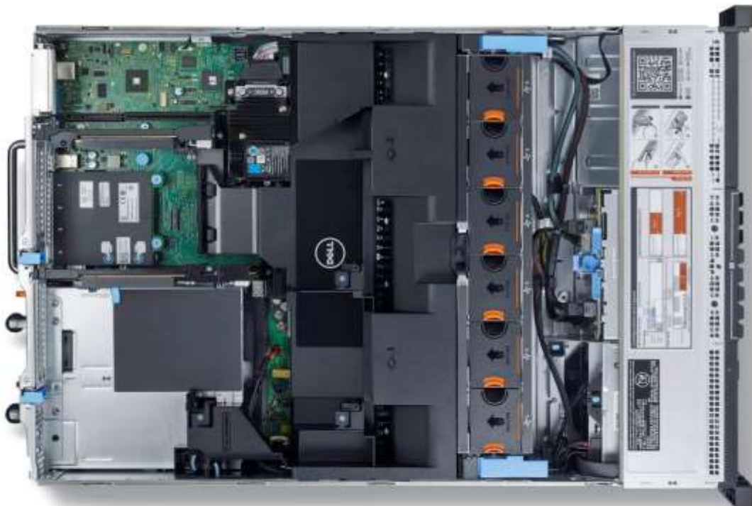
Figure 7. R730 internal chassis view
