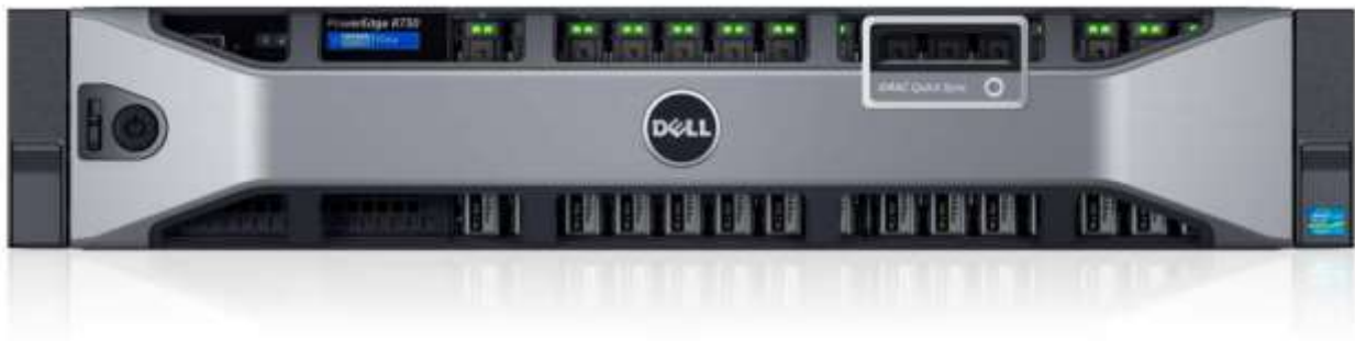
Figure 2. R730 front view (2.5" chassis without bezel)
