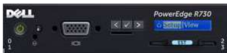
Figure 9. R730 LCD control panel
