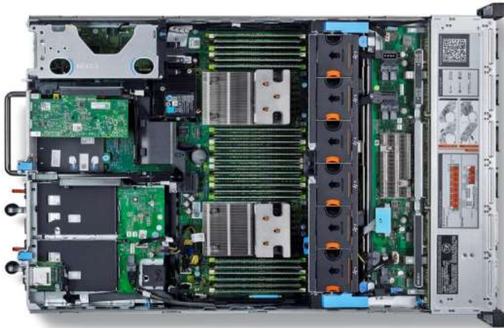
Figure 8. R730xd internal chassis view
