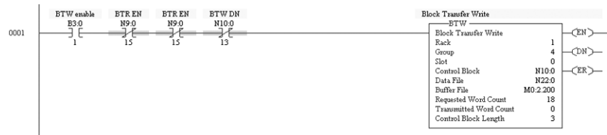
Figure 4.12 SLC 500 Series C, FRN 3.xx and Higher, Example Ladder Logic for Block Transfer Write
