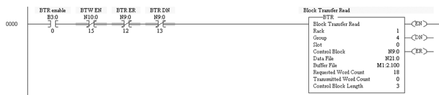
Figure 4.11 SLC 500 Series C, FRN 3.xx and Higher, Example Ladder Logic for Block Transfer Read
