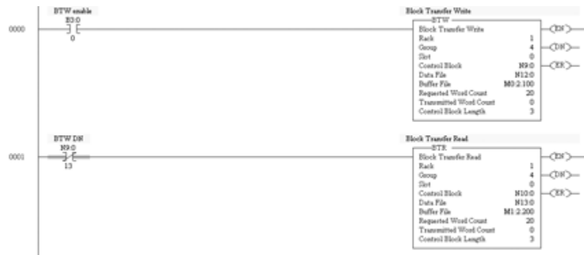
Figure 5.5 SLC 500 Series C, FRN 3.xx and Higher, Example Ladder Logic for Block Transfer Read and Block Transfer Write
