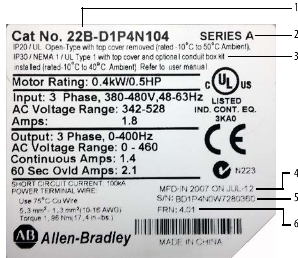
Figure 2 - PowerFlex 40 Drive Data Nameplate Information
