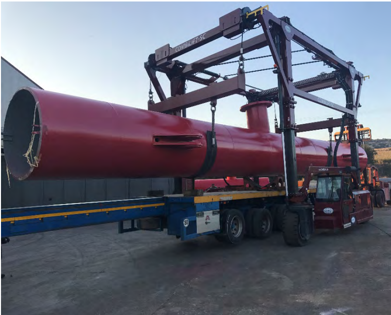
Remote control Telescopic Straddle Carrier SC1260C by Combilift, handling steel structures up to 70tns
