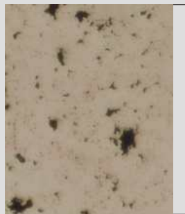
BP25: 8 to 10.5% Sn others < 2% rest Cu, impregnation group 1 (up to +80°C)
