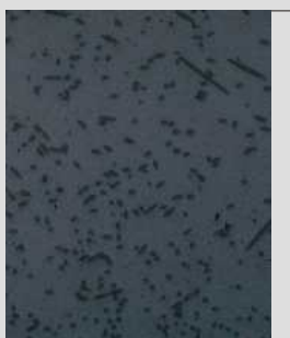
Injection moulded thermoplastic dry bearing material consisting of PAI + Graphite + PTFE
