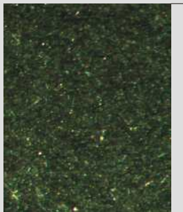
Injection moulded thermoplastic dry bearing material with additives homogeneously mixed in
