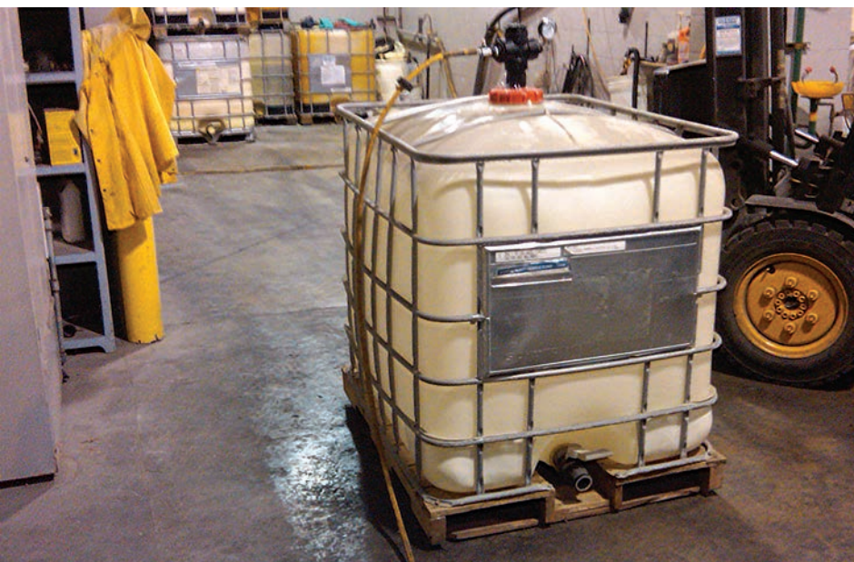
These photos show a tank with almost 2 psi. "We stopped the test, because the two metal straps on top were about to break," the operator said. Always use caution when pressure testing cages!
