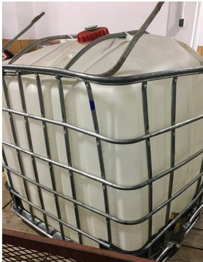
This minibulk fell off a truck's tailgate and incurred significant damage. Note the broken bars of the cage along the top and the bulged and dented poly tank inside the cage.
