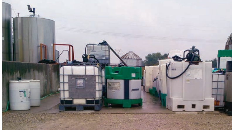
The operational pad holds filled minibulks, while the empties are legally stored outside of containment.
