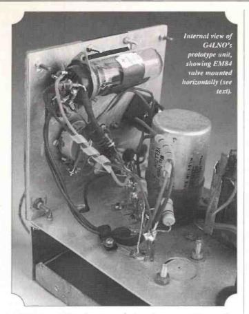
without the use of the spring type tool clips. However, there's nothing to stop you mounting the valve vertically and viewing the 'eye' closing and opening vertically instead of horizontally.
