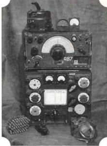
The R1155/T1154 combination. The receiver is on top, along with the 'J' aerial switch (round object on top) and 'bathtub' Morse key. This was complete with locking ring that would hold set on transmit while aircrew bailed out of a stricken aircraft.
