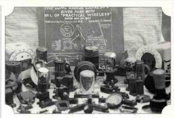
Fig. 1: A typical selection of valves and components available when Ron Ham built his first 'one valver' receiver in 1939 (from the Amberley Chalk Pits Vintage Wireless collection).
