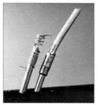
coils and sometimes for connection to the ends. The photograph shows a completed extension butt-joint and the partially made up one.
