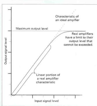
Fig. 1: Characteristic of an r.f. amplifier.
