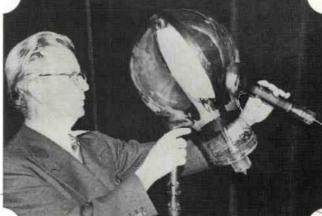
Although Baird demonstrated the two-beam 'Telechrome' colour TV tube (on left), he suggested a suitable arrangement for three colours (centre). Unfortunately his death at the early age of 58 in 1946 robbed television engineering of one of the greatest pioneers. Blue screen Red screen Red screen Rec Thin Mica shee Thin Mica shee Red Red Blue Blue Electron beam 'guns'
