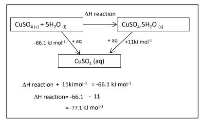
This Hess's law is used to work out the enthalpy change to form a hydrated salt from an anhydrous salt.
