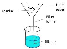
This is gravitational filtration. Use if small amounts of solid are formed.
