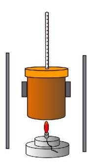
**Example 5**. Calculate the enthalpy change of combustion for the reaction where 0.65g of propan-1-ol was completely combusted and used to heat up 150g of water from 20.1 to 45.5°C
