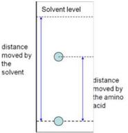
Separation by chromatography depends on the balance between solubility in the moving phase and retention in the stationary phase.
