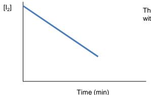
This reaction is zero order with respect to  $I_2$  but  $1^{\rm st}$  order with respect to the propanone and acid catalyst
