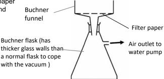
This is vacuum filtration. The apparatus is connected to a water pump which will produce a vacuum. Use if larger amounts of solid are formed.
