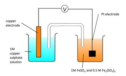
Note: in the electrode system containing two solutions it is necessary to use a platinum electrode and **both** ion solutions must be of a 1M concentration so  $[Fe^{2+}] = 1M$  and  $[Fe^{3+}] = 1M$ .
