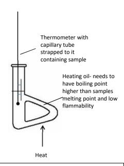
Sometimes an error may occur if the temperature on the thermometer is not the same as the temperature in the actual sample tube.
