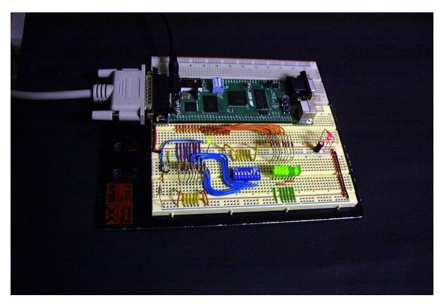
Figure 5.2. Verifying the functionality of the S-Box on a test circuit.
