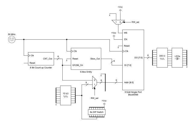
Figure 5.1. Test circuit for performing a field test to the S-Box.
