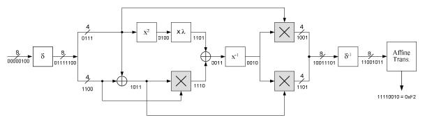
Figure 3.1. A worked example for computing the SubByte operation.
