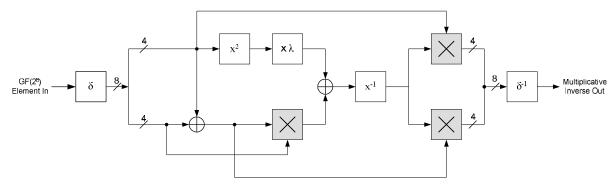
Figure 2.1. Multiplicative inversion module for the S-Box. [1]
