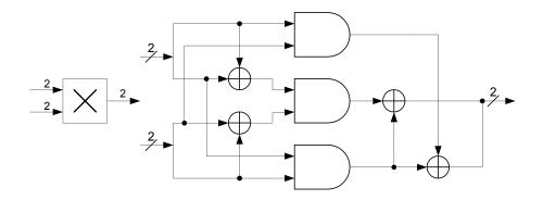
Figure 2.6. Hardware implementation of multiplication in GF(2). [3]
