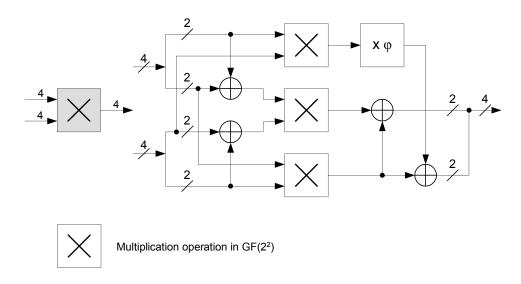
Figure 2.5. Hardware implementation of multiplication in  $GF(2^4)$ . [3]
