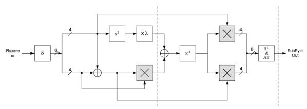
Figure 4.1. Implemented hardware architecture on the FPGA with a 2-layer pipeline.
