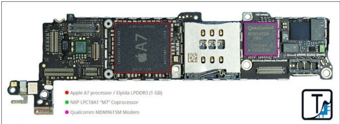
The iPhone 5S teardown image—side one (included with kind permission from TechInsights)
