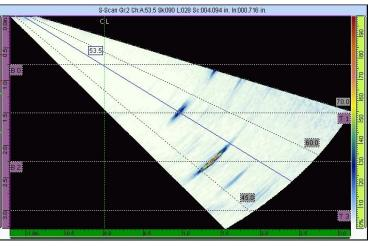
S-scan image of crack signals
